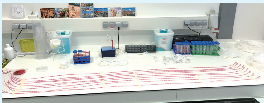
Fig. 3: Horizontally positioned PTFE test specimens after inoculation during the one-hour rest phase
