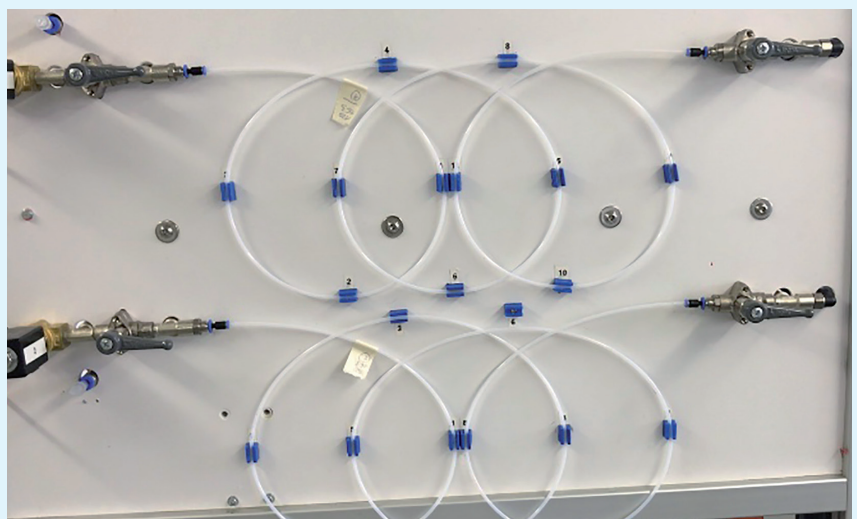
Fig. 4: PTFE test specimens in cleaning stand 2 after Comprex® cleaning
